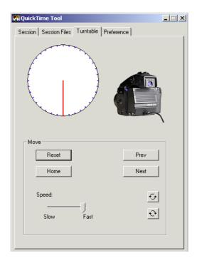
In order to make the turntable move continuously, click on the Clockwise or Counter-clockwise buttons. To stop the turntable, click on one of these buttons again.
